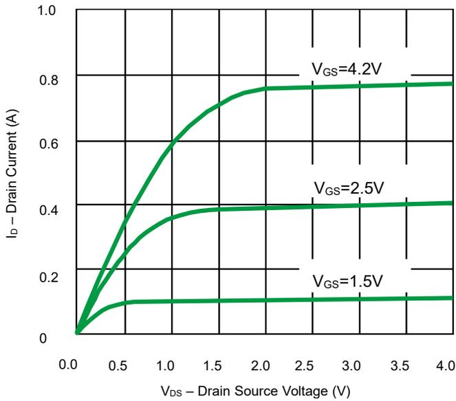
Fig 7. Output Characteristics
