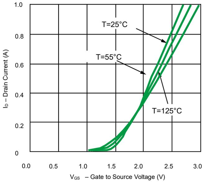
Fig 8. Transfer Characteristics
