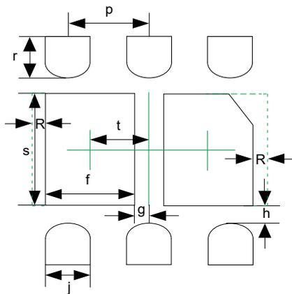
If there is enough place in PCB. It can be mounted with copper along the dotted line in order to optimize thermal design.
